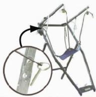
2. Allow the pouch assembly to hang free. Remove safety pins from hinges and replace on "U" frame.
