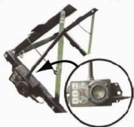
6. Attach the remote receiver to the Winger, insert the electrical plug and turn on the power. Before proceeding test the release. ATTENTION: Refer to the user manual of your remote control electronics for opreating procedures.
