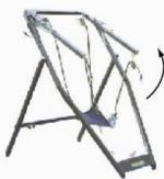
Allow the pouch assembly to hang loose by unhooking the pouch rings from their respective anchor hooks. NOTE: The rubber bands are always crisscrossed when not in use.
