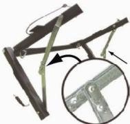
3. Unlock both hinges. WARNING: Care must be taken not to pinch hands or fingers when breaking down the hinges.
