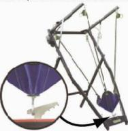
2. Hook the pouches release bolt to the release arm. The release bolt should be positioned as far over as it can go. WARNING: The Winger is now considered armed. Extreme care must be take to prevent accidentally misfiring and injury.
