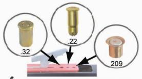
6. OPTIONAL: The Multi-Shot<sup>™</sup>Sound release mechanism accepts three different blanks for simulating a shot sound. Only one can be used at a time. Choose between a 209 primer, .32 or .22 blank. WARNING: The shot sound is extremely loud. Hearing and eye protection must be worn when using the Zinger Winger™ to prevent injury to the user.
