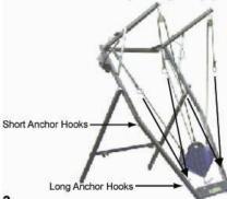
Grasp the rubber above the ring and pull straight down to the anchor hook. For a lesser throw pull to the short anchor hooks; For a greater throw pull to the long anchor hooks. After the lower rubber is hooked up repeat with the top rubber. Place both rings on the same hook. WARNING: Stretch cord carefully. Uncontrolled release can cause severe injury to unprotected bodily parts, particularly eyes
